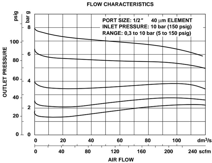
**Ordering Information.** Models listed include ISO G threads, knob adjustment, automatic drain, metal bowl, 40 µm element, relieving diaphragm and 0,3 to 10 bar (5 to 150 psig) outlet pressure adjustment range\* without gauge.
